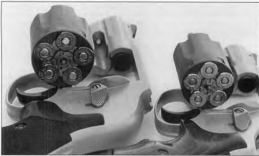
Five beans in the wheel: Both the .44 Special Model 296 and .38 Special Model 337 AirLite Ti revolvers have five-shot cylinders. (above, right) Note lightening "rain gutter" running around the periphery of the trigger guard. Groove on the back of the trigger is not a lightening cut but a function of its manufacture by the MIM process. (right) The steel, serrated ramp-type front sight blade has a black oxide finish which provides high visibility and is held to the barrel shroud by a roll pin.
